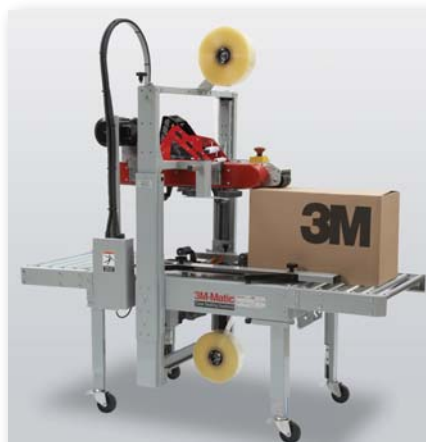
700aks – Especially designed for sealing larger RSCs such as used in the appliance, electronics, and bedding industries. For reliable sealing, the adjustable king size top and bottom belt drive dependably conveys uniform cases up to 25.5" wide by 36" high at up to 40/minute. Includes 72mm tape width 3M™ AccuGlide™ 3 Taping Head.
