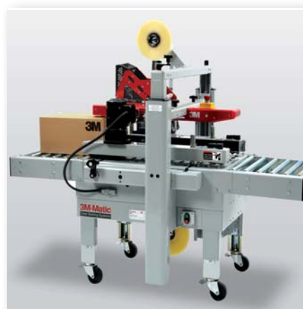
800a – Adjustable side belt drive for a wide range of RSC sizes and weights: lengths of 6" and more; 4.5-21.5" widths; 4.75-24.5" heights. Seals up to 40 cases/minute with 36-48mm wide Scotch® Box Sealing Tapes.
