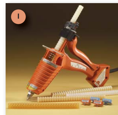
I 3M™ Scotch-Weld™ Hot Melt Applicator EC. Medium volume; variable temperature control. 138
