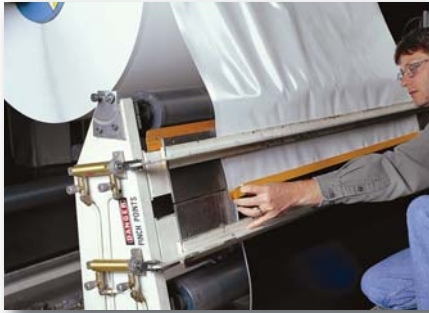
Versatile 3M™ Performance Flatback Tape 2525 provides high visibility for holding many materials, edge banding, and splicing. 311
